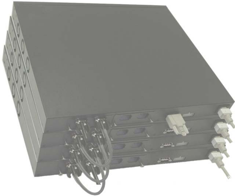
Figure 1-3. Connecting a Stack of Switches
